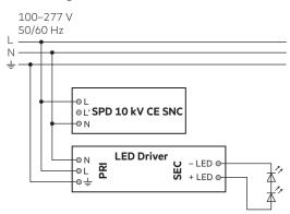
Single-branch wiring with connection of L':
