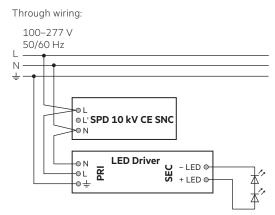
Through wiring with connection of L':
