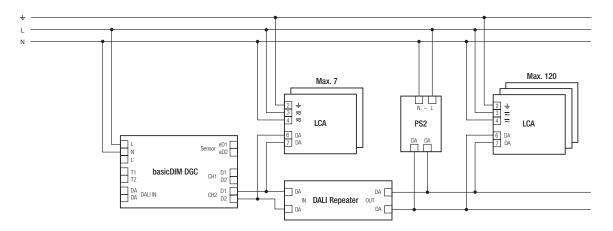
DALI PS1 (24034323), 200 mA, max. 100 additional devices DALI PS2 (28000876), 240 mA, max. 120 additional devices
