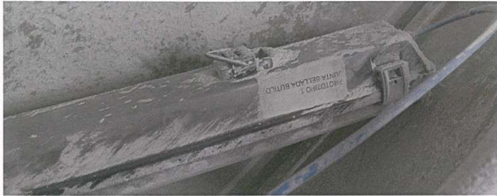
Fig. 5. Enclosure of WATEX fixture after a dust chamber test.
