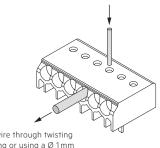
Loosen wire through twisting and pulling or using a Ø 1mm release tool
