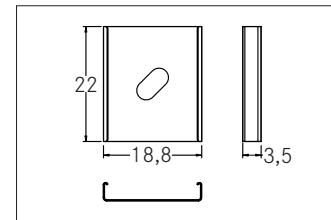
Holder set, alu. Material: Aluminium, dimensions profile: length: 22 mm x width: 18,8 mm x height: 3,5 mm .
