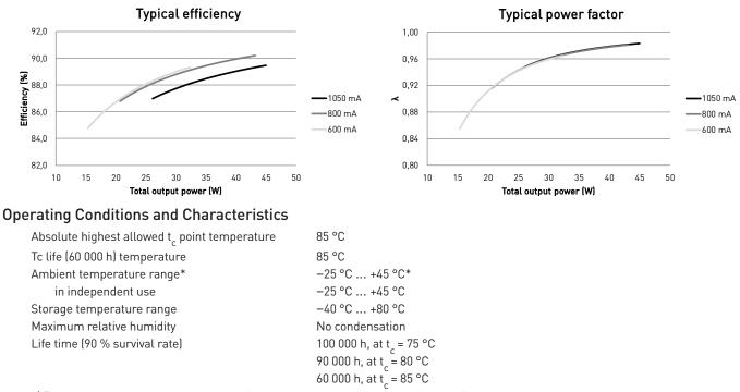
\*) For other than independent use, higher t, of the controlgear possible as long as highest allowed t, point temperature is not exceeded
