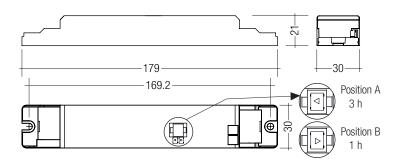
Note: LED Driver supplied with duration link in 3 hours position. Duration link must be set before battery and mains connection. The EM converterLED ST 134 NiCd is supplied without a duration link. The duration is set to 3 hours and cannot be changed.
