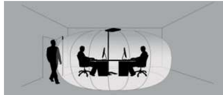
Fig. 11: Detection range of the PULSE HFMD.
