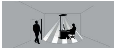
Fig. 12: Detection range of the PULSE PIR.
