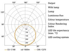
8,5 W Yes, STEINEL LED system LED cannot be replaced 700 lm 3000 K = 82 50000 h Passive Thermo Control
