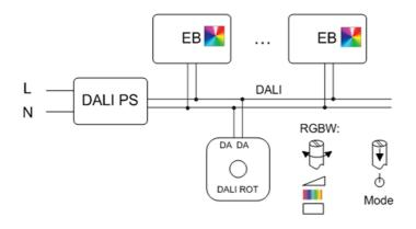
application: colour control RGB+W and dimming
