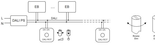
application: switch and dim with DALI ROT module
