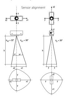
Example for light and motion detection area at height of 1.7 m:
