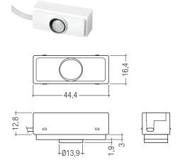
Ultra-compact luminaire mounted sensor for ambient light and detection of movement.
