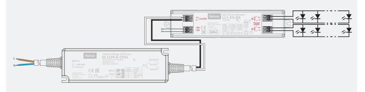
Note: Output voltage is PWM modulated and equal to CV driver output voltage
