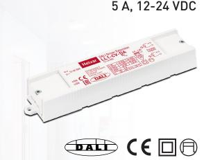
The LL1-CV-DA DALI dimmable extension unit is designed to be used with the Helvar constant voltage LED drivers, creating controllable solutions for decorative lighting. It enables the use of DALI control in constant voltage (12 / 24 V) lighting applications.
