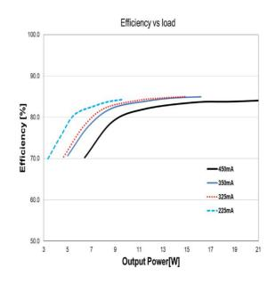
OT FIT 18 CS PC Typical Efficiency vs. Load
