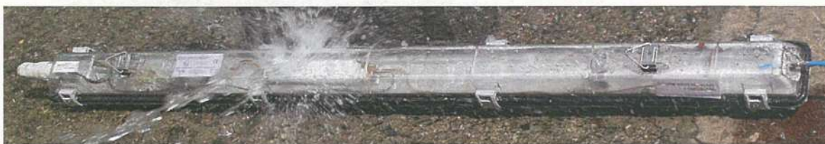
Fig. 6. Enclosure of WATEX fixture after a water test.
