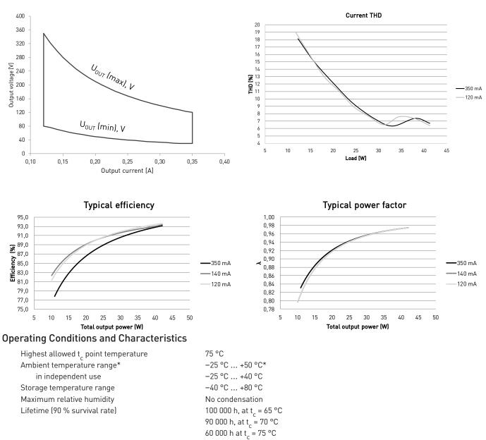
\*) For other than independent use, higher t<sub>a</sub> of the control gear possible as long as highest allowed t<sub>a</sub> point temperature is not exceeded
