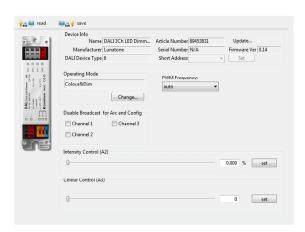
Switching between operating modes can also be done with the help of the DALI-command SET OPERATING MODE (IEC 62386-102 Ed.2). When changing the operating mode the number of used DALI-addresses can change as well and this requires a new addressing
