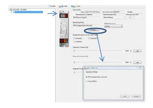
In addition, on the same page the PWM-frequency can be selected and basic control elements for testing each operating modes are available (3 sliders for the level of each channel in operating mode DT6 and slider for level and colour in the operating mode Colour&Dim). Furthermore the broadcast control can be deactivated for each channel individually.
