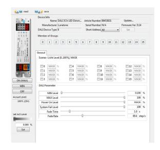
For each address the group membership can be set as well as scene values and DALIparameters. In Colour&Dim operating mode, all values assigned to channel 2 are representing colours.
