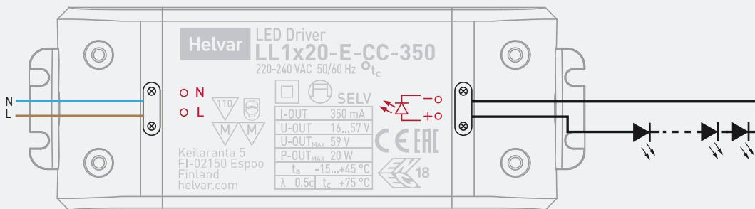
Note: Not suitable for load side switching operation.
