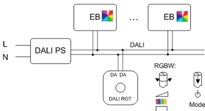
application: colour control RGB+W and dimming
