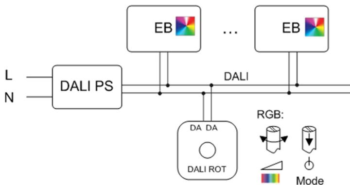
application: colour control RGB + dimming
