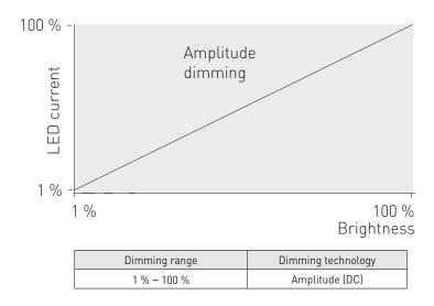
LC45SE-DA-600-1050-LOOP driver implements amplitude dimming technology across whole dimming range. Amplitude dimming offers the best available technology for dimming the light output in an accurate and flicker-free way to ensure high quality lighting in even the most demanding situations such as camera recording applications. Amplitude dimming technology complies with IEEE 1789-2015 recommendations of current modulation to mitigate health risks to viewers.
