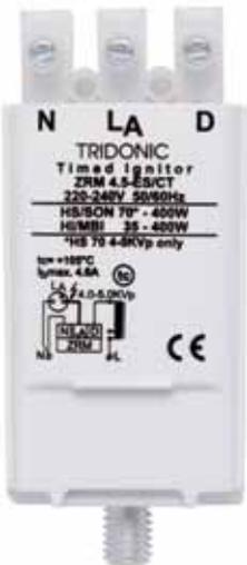
100 % compliance with the tolerance limits of the ignition pulse is guaranteed because ignition characteristics do not depend on external components. Furthermore, the high voltage is applied exclusively to the ignitor and light source without placing a high-voltage load on the choke. This extends the choke's service life considerably.
