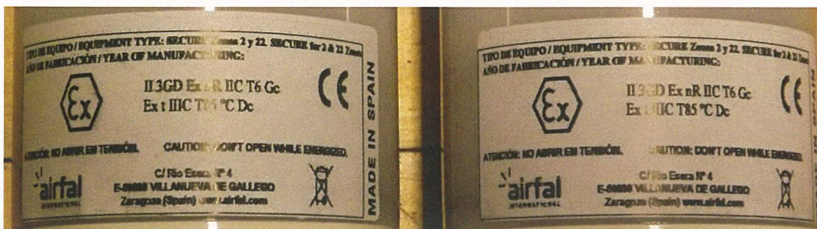
Picture 3. Determination of the type of construction of tested luminaries
