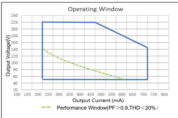
It's important to set output current (AOC value) according to LEDs voltage, make sure the power is within 100W +5%
